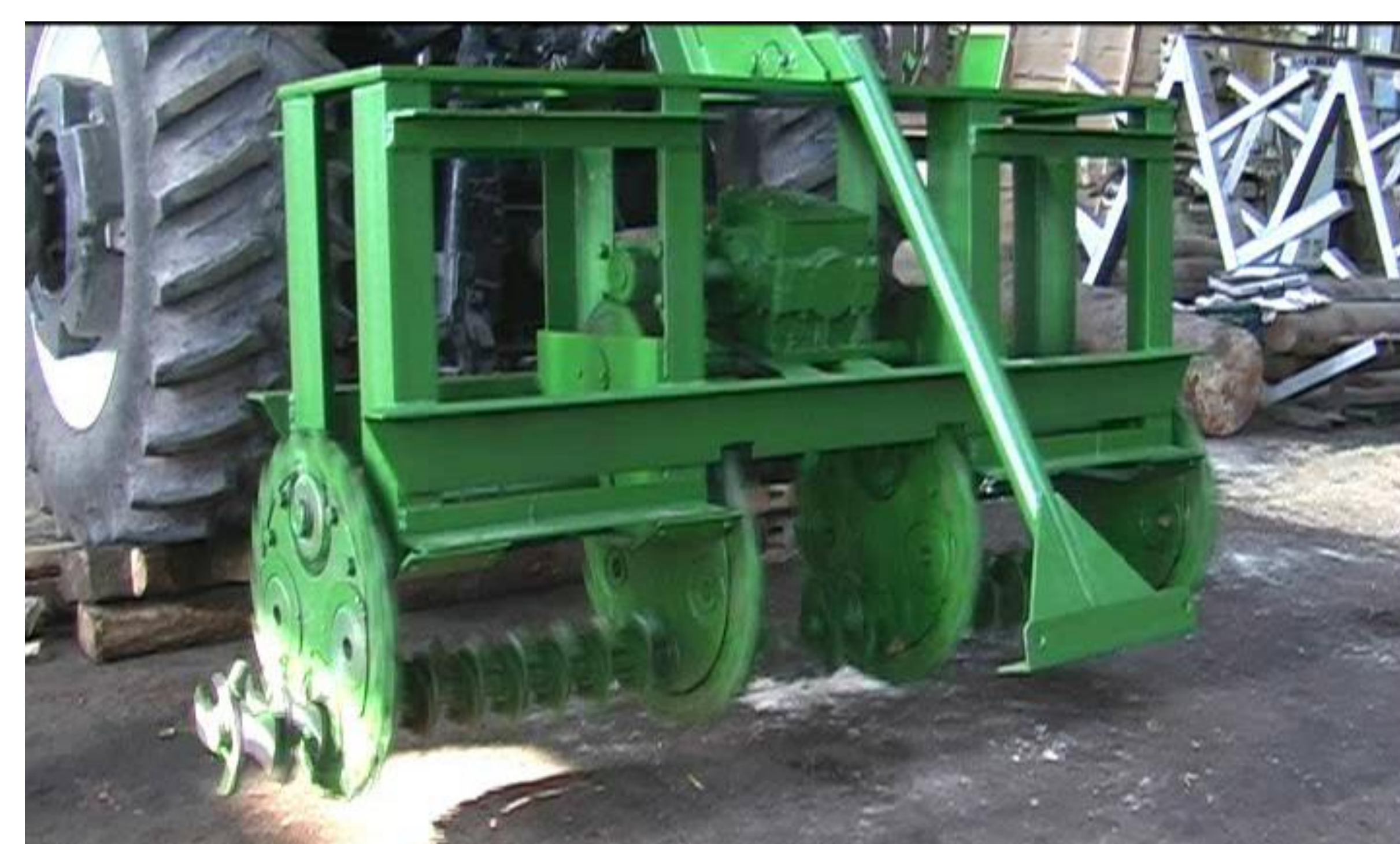
Fig. 1. Soil-milling device PMS-70. Mechanical drive (1), loosening knife (2), reducer rack (3), rotary milling ripper (4), topsoil passive plow (5).
